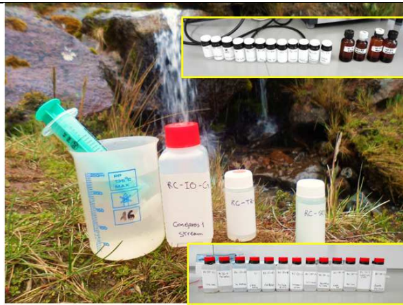
Figure 10: Samples taken for major ions, trace elements and stable isotopes in Stream 1. In frames, group of samples once in the laboratory of the TU Darmstadt.
