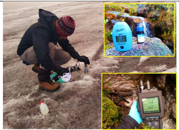
Figure 11: Measuring of physico-chemical parameters and sampling on the Conejeras glacier for the sample "Glacier melting – GM". In detail, colorimeter alkalinity meter and multiparameter for pH, conductivity and temperature.
