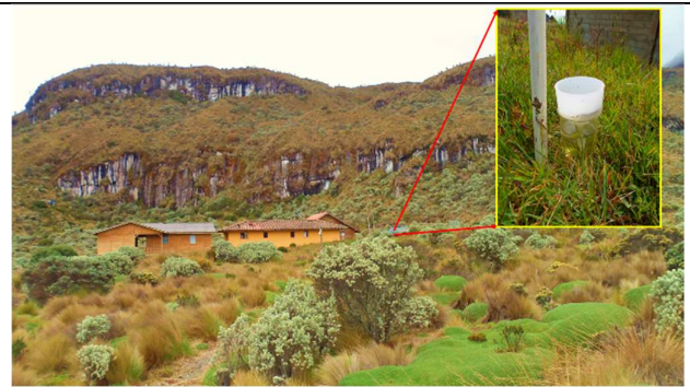
Figure 9: Collector Erlenmeyer used to store the precipitation in Precip. 8 next to the Cisne hut.
