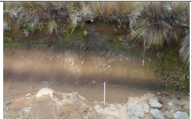
Figure 3: Typical soil profile showing layers of organic matter alternated with volcanic ashes. Scale equals 50 cm
